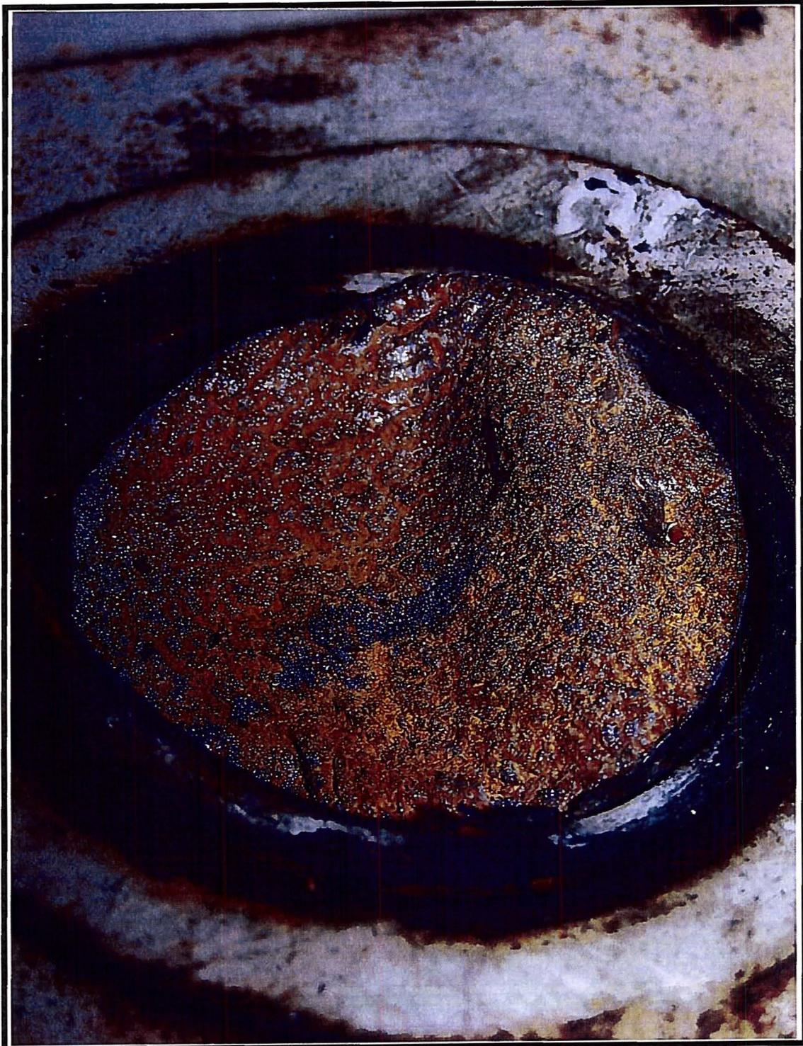
**FIGURE 4:** Picture of pin half still in place on scissor lift.
