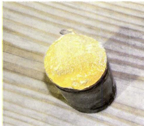
Photo 8 – Pivot Shaft Fracture Surface
