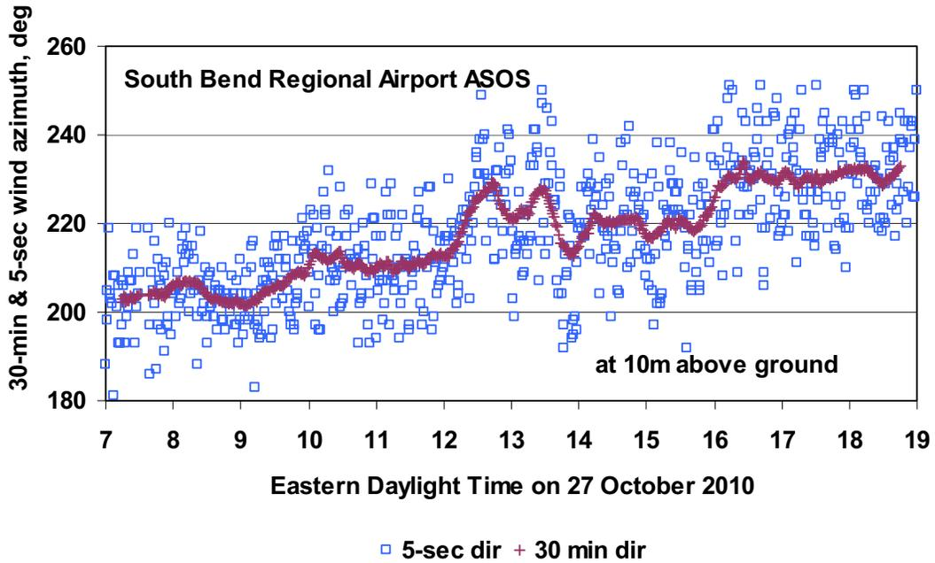
Figure 3c. Thirty-minute mean wind azimuth and 5-second azimuths from South Bend Regional Airport.
