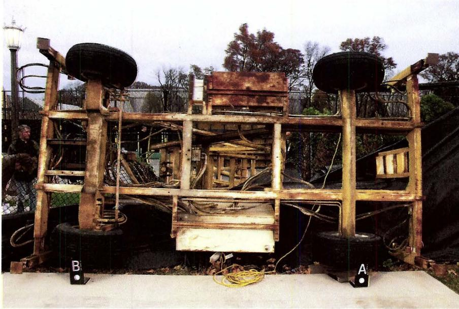
Photo 1 - Lift in Tipped Condition Showing Outrigger Position
