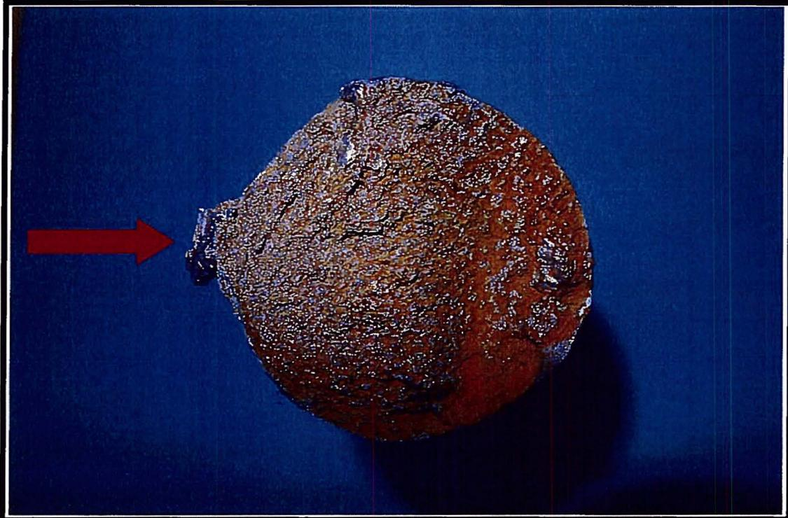
**FIGURE 3:** End view of fracture showing weld metal (arrow).
