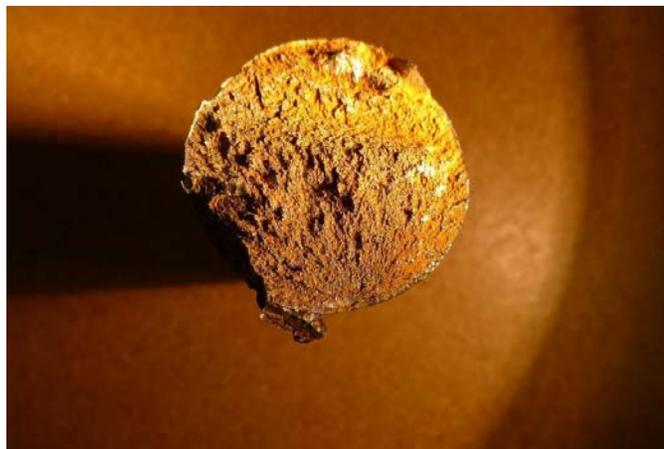
Based on his examination of the fracture surface, Biery concluded that “[t]he pin most likely broke due to impact of the platform and scissor assembly with the ground.” Because the fracture did not preexist the accident, it was also excluded as a cause.
