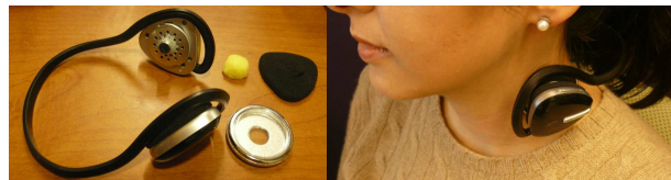
Figure 1. The BodyScope prototype. It consists of a Bluetooth headset, a microphone (embedded in the headset), and the chestpiece of a stethoscope.
