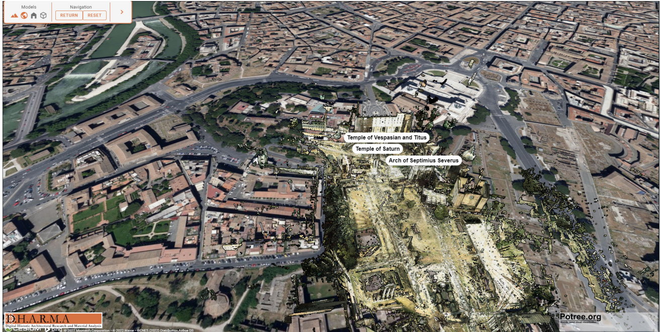
Figure 2. The aerial view of our visualization of the Roman Forum shows the point cloud data overlaid with a Cesium global map, which provides contextual information. The control panel is on the top-left side.
