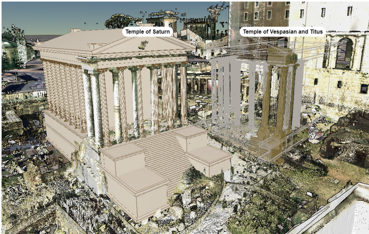
Figure 4. The reconstructed fine model of Temple of Saturn and the coarse mesh model with a wireframe of Temple of Vespasian and Titus. Both models are overlaid over the point cloud as the context.
