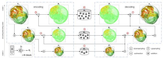
Figure 1: Employing the Laplacian pyramid, ECNR decomposes a volume into blocks in terms of their low-resolution content (coarsest scale) and residuals (finer scales). A three-scale (s = 3) example with the simplified 3D version (i.e., the temporal dimension is omitted) is sketched. A group of MLPs encodes all blocks at the same scale.
