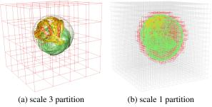
Figure 2: At each scale, the encoding target is split into equal-sized blocks, and only effective blocks with large residual values (shown in red bounding boxes) are processed.
