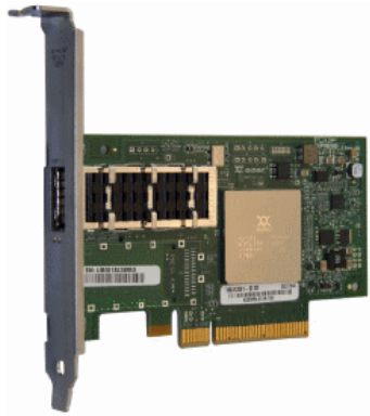
Adapter card: Processing node's link to interconnect
