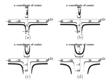
**Fig. 3.** *x*-coordinates of centers of stability region's boundaries versus  $a\Delta t$  for CWC (star) and WCW (dot) schemes: (a)  $d\Delta t = 1.0$ ; (b)  $d\Delta t = 2.0$ ; (c)  $d\Delta t = 4.0$ ; (d)  $d\Delta t = 6.0$ .
