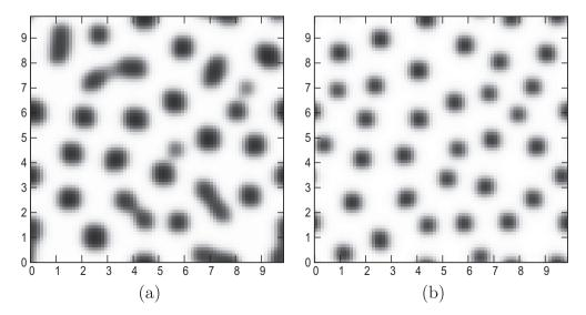
**Fig. 6.** Patterns generated by WCW scheme simulations on an 80 × 80 grid up to t = 30 with (a)  $\Delta t = 6.25 \times 10^{-3}$  and (b)  $\Delta t = 3.125 \times 10^{-3}$ . The parameters of the system are the same as those used in Fig. 5.
