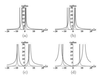
**Fig. 4.** Radius of stability region versus  $a\Delta t$  for CWC (solid) and WCW (dashed) schemes: (a)  $d\Delta t = 1.0$ ; (b)  $d\Delta t = 2.0$ ; (c)  $d\Delta t = 4.0$ ; (d)  $d\Delta t = 6.0$ .
