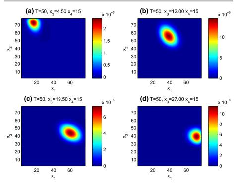
Fig. 11 Distribution of molecular species A and B with  $E_A = 4.5$ , 12, 19.5, 27 and  $E_B = 15$ . Numerical solutions of (67) using the KrylovIIF2-WENO scheme. Final time T = 50.  $\Delta t = 0.1$ . The numbers of spatial grid points are  $N_A = 40$ ,  $N_B = 40$ ,  $N_{E_A} = 20$ ,  $N_{E_B} = 20$
