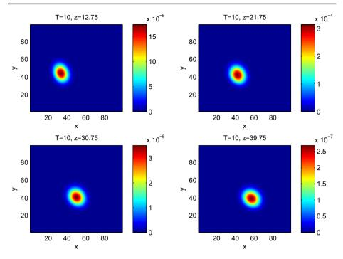
**Fig. 7** Distribution of molecular species A and B with  $E_A=12.75, 21.75, 30.75, 39.75$ . Numerical solutions of (63) using the AcIIF2-WENO scheme with Krylov subspace approximations. Final time T=10.  $\Delta t=0.017$ . The numbers of spatial grid points are  $N_A=120, N_B=120, N_{E_A}=60$
