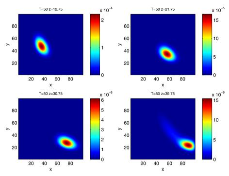
Fig. 5 Distribution of molecular species A and B with  $E_A=12.75, 21.75, 30.75, 39.75$ . Numerical solutions of (63) using the KrylovIIF2-WENO scheme. Final time T=50.  $\Delta t=0.017$ . The numbers of spatial grid points are  $N_A=120, N_B=120, N_{E_A}=60$
