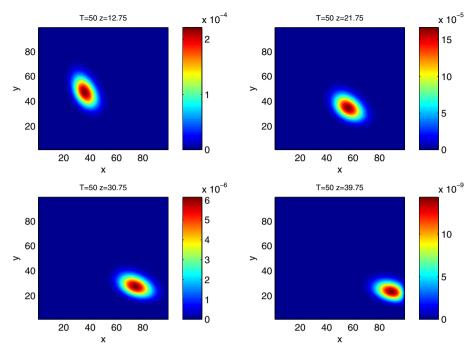
Fig. 8 Distribution of molecular species A and B with  $E_A = 12.75, 21.75, 30.75, 39.75$ . Numerical solutions of (63) using the AcIIF2-WENO scheme with Krylov subspace approximations. Final time T = 50.  $\Delta t = 0.017$ . The numbers of spatial grid points are  $N_A = 120$ ,  $N_B = 120$ ,  $N_{E_A} = 60$
