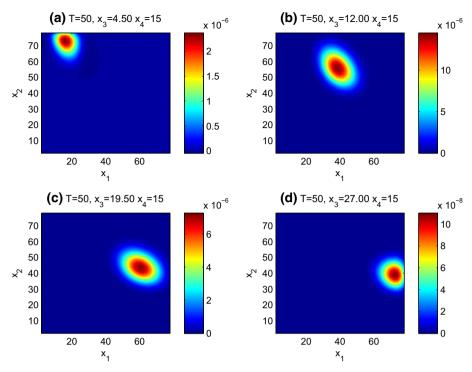
Fig. 14 Distribution of molecular species A and B with  $E_A = 4.5$ , 12, 19.5, 27 and  $E_B = 15$ . Numerical solutions of (67) using the AcIIF2-WENO scheme with Krylov subspace approximations. Final time T = 50.  $\Delta t = 0.1$ . The numbers of spatial grid points are  $N_A = 40$ ,  $N_B = 40$ ,  $N_{E_A} = 20$ ,  $N_{E_B} = 20$
