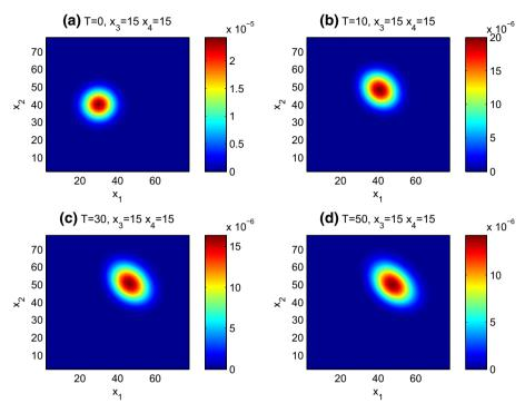
Fig. 15 Distribution of molecular species A and B with  $E_A=15$  and  $E_B=15$ , at time T=0, 10, 30, 50. Numerical solutions of (67) using the AcIIF2-WENO scheme with Krylov subspace approximations.  $\Delta t=0.1$ . The numbers of spatial grid points are  $N_A=40$ ,  $N_B=40$ ,  $N_{E_A}=20$ ,  $N_{E_B}=20$
