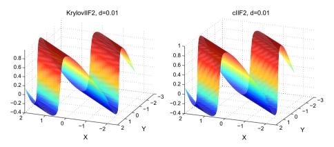
Fig. 3 Numerical solutions of nonlinear viscous Burgers' equation on a  $80 \times 80$  mesh by the Krylov IIF2-WENO scheme and the cIIF2-WENO scheme. Time  $T=5/\pi^2$ . Left picture result of Krylov IIF2-WENO; right picture result of cIIF2-WENO
