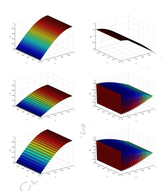
Figure 3.5: Justification for the necessity of checking the signs of  $u_{ij}^{new}$  and  $v_{ij}^{new}$  in the local solver in Section 2.1 and 2.2. The exact solution is  $\phi(x, y) = \sin(\frac{\pi}{2}x)$ .  $\phi_h$  is computed when the signs of  $u_{ij}$  and  $v_{ij}$  are checked (top), when the signs are not checked (middle), and when the signs are not checked and the pure DG local solver is used (bottom). Left:  $\phi_{ij}$ ; Right:  $u_{ij}/h$ . n = 1/h = 40.
