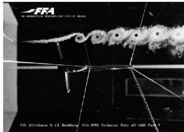
Figure 12: Photograph of the cross-section of the tip vortices from a two-bladed wind turbine that was visualized in a wind tunnel experiment[?].
