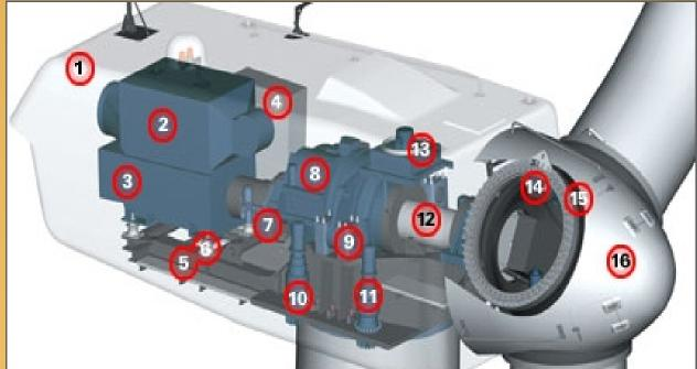
1. Nacelle 2. Heat Exchanger 3. Generator 4. Control Panel 5. Main Frame 6. Impact Noise Insulation 7. Hydraulic Parking Brake 8. Gearbox 9. Impact Noise Insulation 10. Yaw Drive 11. Yaw Drive 12. Rotor Shaft 13. Oil Cooler 14. Pitch Drive 15. Rotor Hub 16. Nose Cone
