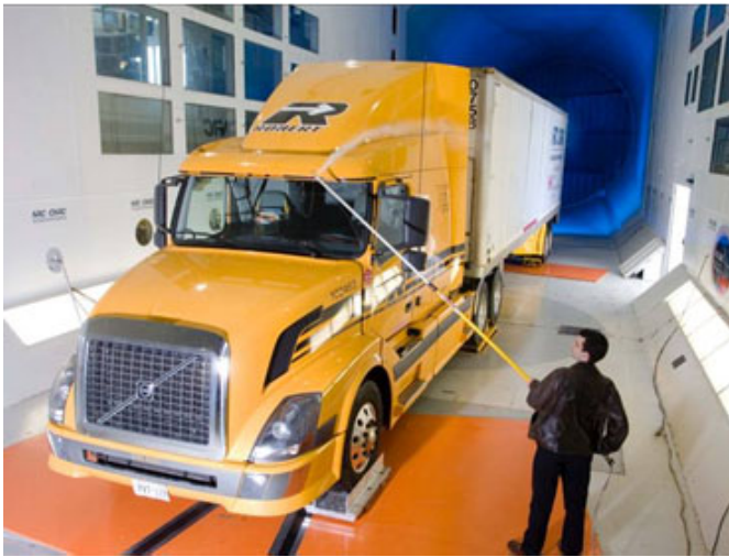
Figure 24 – Full-scale tractor-trailer testing in the NRC 9 m x 9 m Wind Tunnel
