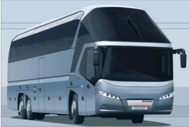
Figure 22 – German-designed intercity bus with C_D \approx 0.35 .
