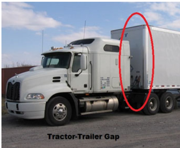
Figure 13 – Typical tractor-trailer gap
