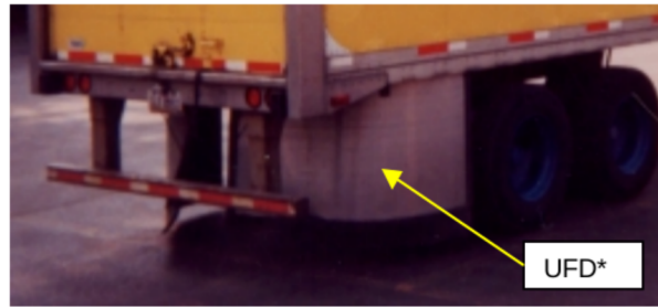
Figure 20. Photograph of the undercarriage flow treatment device installed on the aft trailer undercarriage.
