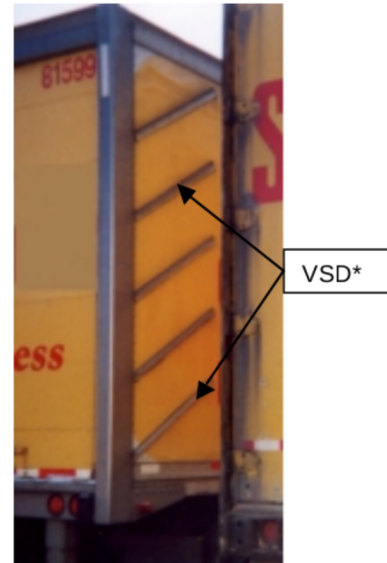
Figure 17. Photograph of the vortex strake trailer base treatment device installed on the aft portion of the trailer.
