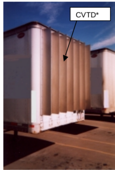
Figure 12. Photograph of the cross flow vortex trap gap treatment device installed on the trailer front face.
