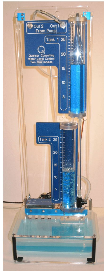
Figure 1 The Coupled-Tank Experiment
