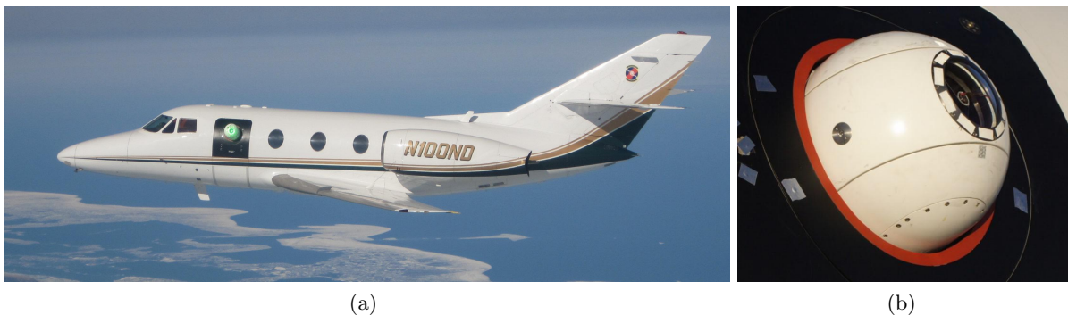
Figure 1. Photographs of AAOL-T hardware during testing. (a) The sensor turret integrated on the aircraft receiving the green test beam in flight. (b) A closer look at the AAOL-T turret integrated on laboratory aircraft.
