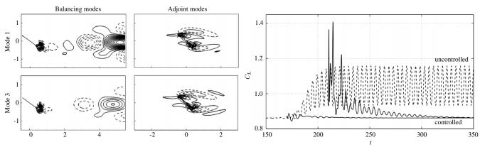
Fig. 8 Use of balanced POD analysis for feedback stabilization of the unstable wake behind a flat plate (Re = 100,  $\alpha = 35$  deg) [93]. First and third balancing and adjoint modes are shown on the left. Baseline lift history is shown with a dashed line, and controlled cases with different initiation times of feedback control using the balanced-POD-based reduced-order model are plotted in solid lines on the right. Reprinted with permission from Cambridge University Press.
