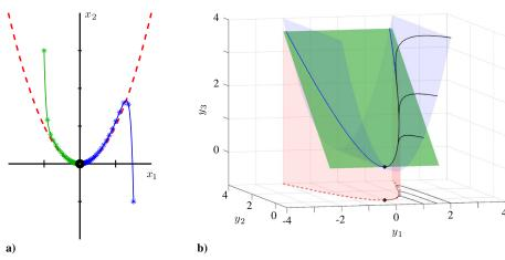
Fig. 11 Example illustrating how the nonlinear system in Eq. (53), shown in Fig. 11a, may be transformed into the linear system in Eq. (54), shown in Fig. 11b, through an appropriate choice of measurements y of the state x. In this case, the measurement subspace given by  $(y_1, y_2, y_3) = (x_1, x_2, x_1^2)$  provides a matrix representation K of the Koopman operator. Modified from [142].
