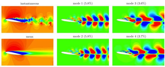
Fig. 6 POD analysis of turbulent flow over a NACA0012 airfoil at Re = 23,000 and  $\alpha = 9$  deg. Shown are the instantaneous and time-averaged streamwise velocity fields and the associated four most dominant POD modes [73,74]. Reprinted with permission from Springer.
