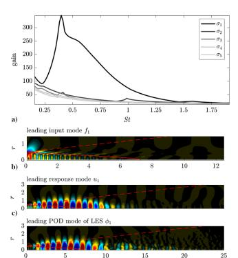
Fig. 16 Resolvent analysis of a turbulent jet mean flow. The gains  $\sigma$  of the five leading axisymmetric resolvent modes over Strouhal number are reported in Fig. 16a. As an example, the pressure component of the leading input mode  $f_1$  for St=0.5 is shown in Fig. 16b. The corresponding response  $u_1$  shown in Fig. 16c closely resembles the leading POD mode  $\phi_1$  deduced from LES data in Fig. 16d.
