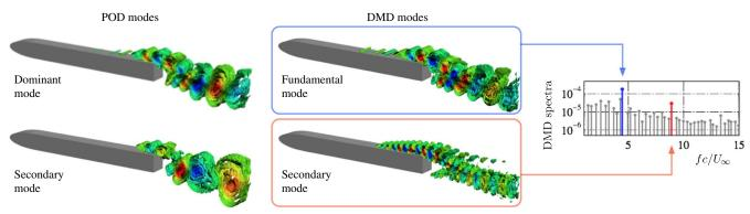
Fig. 10 Comparison of POD and DMD modes for separated three-dimensional turbulent flow over a flat-plate wing with synthetic-jet actuation on the top surface [134]. The fundamental and secondary DMD modes correspond to the actuation frequencies of 4.40 (blue) and its superharmonic (red). Reprinted with permission from J. Tu.
