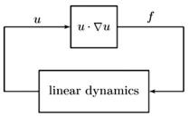
Fig. 14 Schematic of a divergence-free projection of the resolvent formulation of the incompressible Navier–Stokes equations, showing the nonlinear term f providing input forcing to the linear dynamics (described by the resolvent operator), with velocity output, u [i.e., q' in Eq. (58)] [195]. Reprinted with permission from AIP Publishing.
