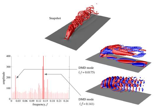
Fig. 9 Snapshot of jet-in-crossflow data used for DMD [105], shown with  $\lambda_2$  contour in the top plot. The frequency and amplitude of the DMD modes are shown in the bottom left plot, whereas the bottom right figures show the modes corresponding to (dimensionless) frequencies of 0.0175 and 0.141, visualized with contours of streamwise velocity. Reprinted with permission from Cambridge University Press.
