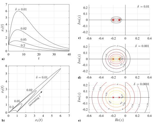
Fig. 5 Representations of a) example of transient growth caused by increasing level of nonnormality from decreasing  $\delta$ , b) trajectories of  $x_1(t)$  vs  $x_2(t)$  exhibiting transient growth, and c-e) pseudospectra expanding for different values of  $\delta$ .  $\epsilon$  pseudospectra are shown with values of  $\log_{10}(\epsilon)$  placed on the contours, and stable eigenvalues are depicted with  $\times$ .
