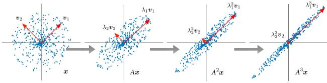
Fig. 2 Collection of random points (vectors x) stretched in the direction of the dominant eigenvector  $v_1$  with iterative operations  $A^k$  for matrix A, which has eigenvalues of  $\lambda_1 = 1.2$  and  $\lambda_2 = 0.5$ .
