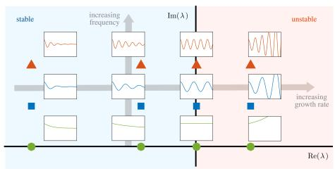
Fig. 3 Dynamic response of a linear system characterized by the eigenvalues (stable:  $Re(\lambda) < 0$ , and unstable:  $Re(\lambda) > 0$ ). Location of example eigenvalues  $\lambda$  are shown by the symbols with corresponding sample solutions  $\exp(\lambda t)$  in inset plots.
