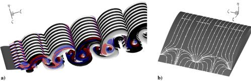
Fig. 12 Three-dimensional short-wavelength instability mode determined from a global stability analysis for a NACA 4415 airfoil at Re = 500 and  $\alpha = 20$  deg: a) streamwise vorticity  $\omega_{\zeta}$  isosurface of the short-wavelength eigenmode, and b) the corresponding wall streamlines, superposed upon the time-periodic base state [169]. Reprinted with permission from Cambridge University Press.
