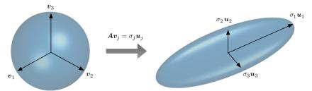
Fig. 4 Graphical representation of singular value decomposition transforming a unit radius sphere, described by right singular vectors  $v_j$ , to an ellipse (ellipsoid) with semiaxes characterized by the left singular vectors  $u_j$  and magnitude captured by the singular values  $\sigma_j$ . In this graphical example, we take  $A \in \mathbb{R}^{3\times 3}$ .
