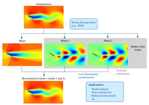
Fig. 1 Modal decomposition of two-dimensional incompressible flow over a flat-plate wing [25,26] (Re = 100 and  $\alpha = 30$  deg). This example shows complex nonlinear separated flow being well represented by only two POD modes and the mean flowfield. Visualized are the streamwise velocity profiles.
