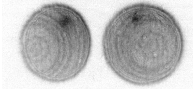
Figure 7: Unthresholded inverted-color upstream and downstream spot patterns for focused Malley probe at a C/L ratio of 20%.
