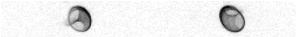
Figure 8: Unthresholded inverted-color upstream and downstream spot patterns for focused Malley probe at a C/L ratio of 5%.
