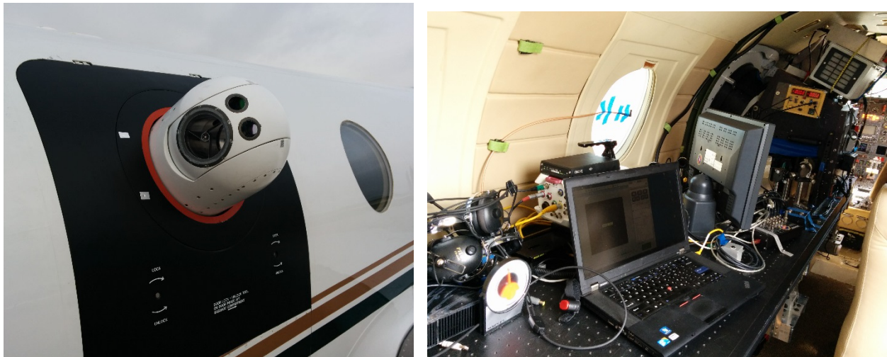
Figure 2. The AAOL turret installed on AAOL-T, left and the instrumented optical bench, right.
