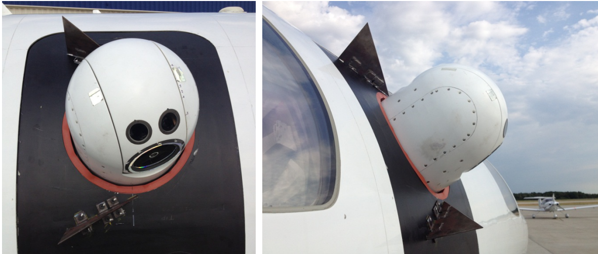
Figure 4: The vortex generators mounted on the AAOL. The flow goes from right to left.
