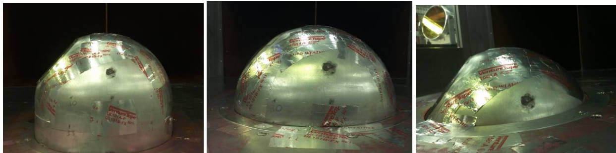
Figure 4. Tested turret geometries with a flat-aperture: a full turret (left), a hemisphere (middle) and a partially-protruding hemisphere (right).
