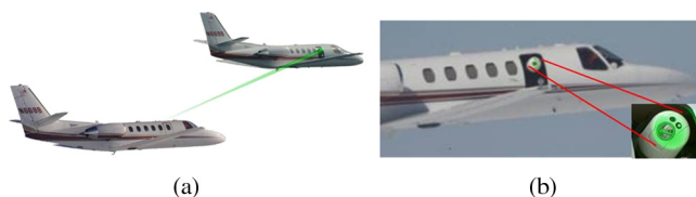
Fig. 6 Airborne Aero-Optics Laboratory (left) schematic of the two citations flying in formation; (right) picture taken during a flight test, note laser on the turret.
