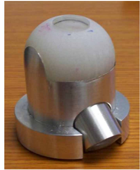
Fig. 4 Conformal window turret for optical WFS measurements (dimensions in mm)
