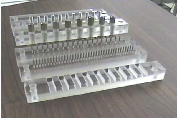
Figure 4. Pin configurations and, in the closest configuration, the cavity configuration.
