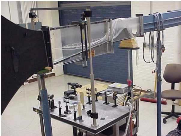
Figure 9. WCSL Facility with Malley-Probe Set Up on the Optical Bench.
