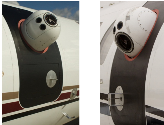
Figure 2. The AAOL turret, as a full hemisphere-on-cylinder turret, left and a hemisphere-only turret, right.
