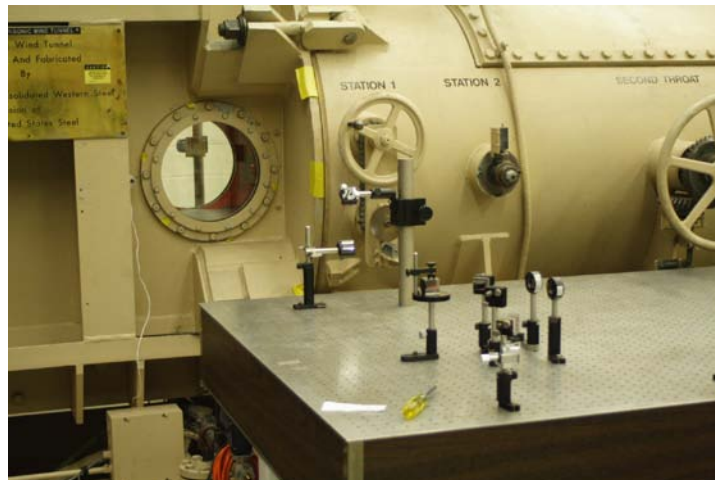
Figure 1. Top: Schematic of the US Air Force Academy Trisonic Wind Tunnel. Bottom: The test section with 1-ft-diameter optical windows.
