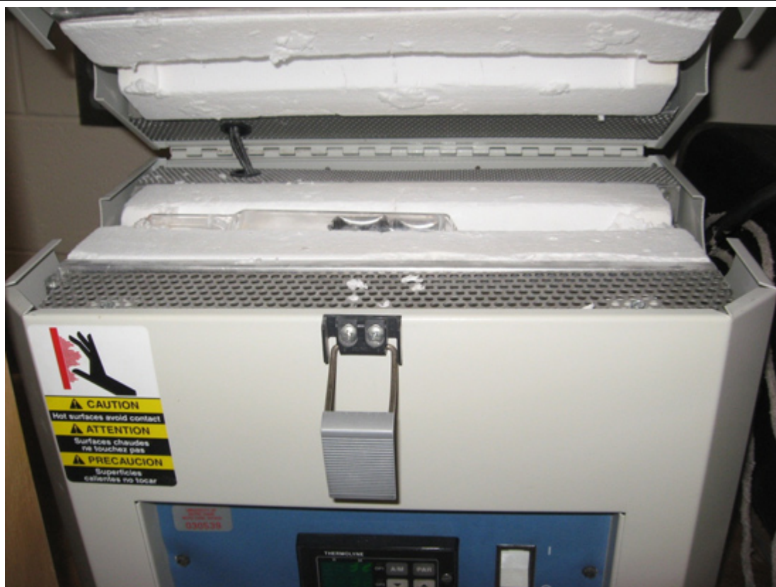
Figure 8. Schematic representation of Placing Loaded Fused Silica Tubes in Furnace.
