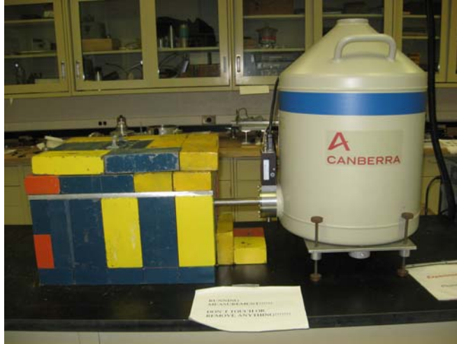
Figure 1: The lead castle and Germanium detector set-up located in the NSL.
