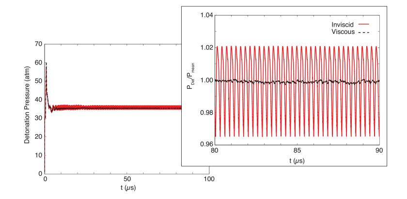
The addition of physical viscosity delays the onset of the initial appearance of instability. The small variations present in the viscous case are due to the detonation traversing a non-uniform grid and will be reduced as the tolerance of the WAMR is reduced.
