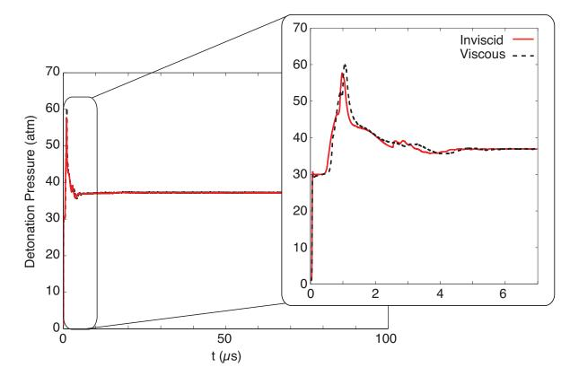
The viscous case smooths the initialization; due to this slightly weaker shock, it takes longer to ignite the detonation. This delay increases the von Neumann spike. Additionally, the viscosity causes the detonation to take longer to relax to steady state.
