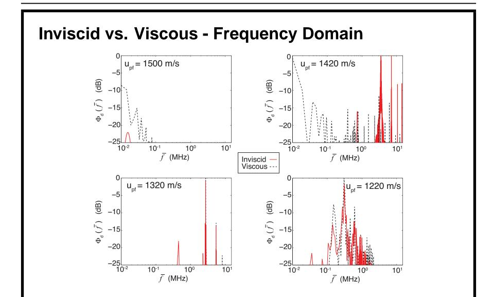
The inviscid case under goes a transition to instability before the viscous case; it also enters the dual mode oscillations before the viscous case. At the lower piston velocities the inviscid case appears to be chaotic sooner.
