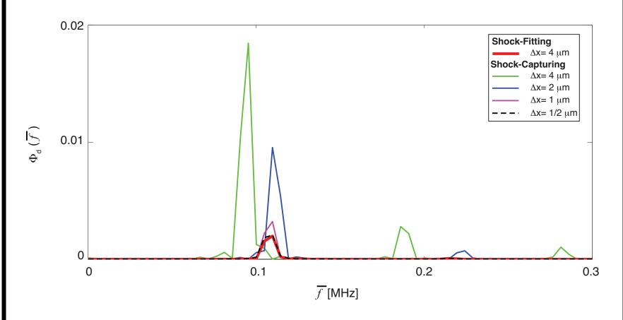
Only when  $\Delta x=1/2~\mu{\rm m}$  is used does the PSD of shock-capturing become nearly indistinguishable with that of shock-fitting.
