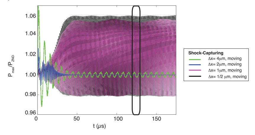
Using the same grid size as shock-fitting ( $\Delta x=4~\mu{\rm m}$ ), shock-capturing misses the essential dynamics.
