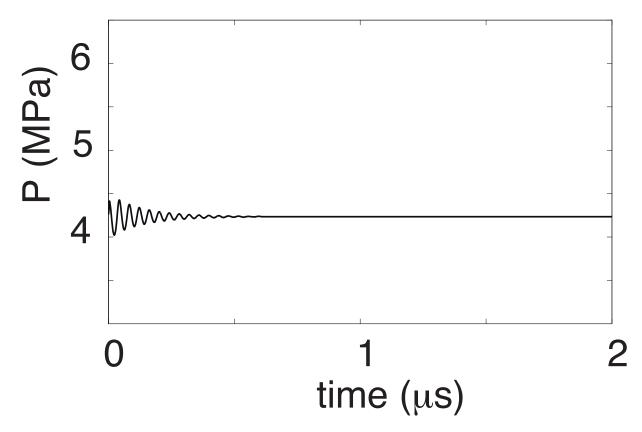
At Higher Activation Energy, Fundamental Harmonic Due to Balance Between Reaction and Advection Between Lead Shock and End of Reaction Zone:
