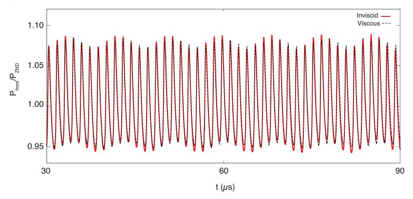
Viscosity still decreases the amplitude of oscillation, though the effect is reduced compared to higher overdrives.
