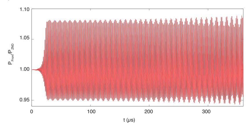
As the overdrive is lowered, multiple frequencies appear, and the amplitude of the oscillations continues to grow. These multiple frequencies persist at long time.
