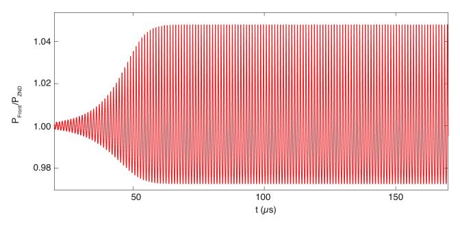
A single fundamental frequency oscillation occurs at a frequency of  $0.97\ MHz$ . This frequency agrees with the experimental observations of Lehr (*Astro. Acta*, 1972).
