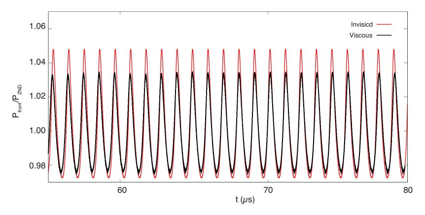
The addition of viscosity has a stabilizing effect, decreasing the amplitude of the oscillations. The pulsation frequency relaxes to  $0.97\,\mathrm{MHz}$ .
