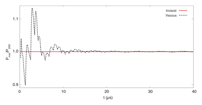
For high enough overdrives, the detonation relaxes to a steady propagating wave in the inviscid case as well as in the diffusive case.
