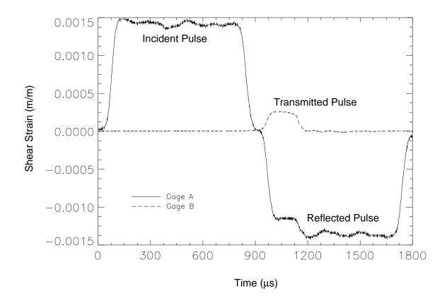
Shear strain in the specimen:
