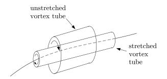
Figure 7.9: Increase in vorticity due to stretching of a vortex tube.
