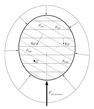
Figure 7.7: Isobars and isochores, center of mass G, and center of pressure for a baroclinic fluid.
