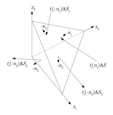
Figure 4.4: Sketch of tetrahedral element for stress analysis on an arbitrary plane.
