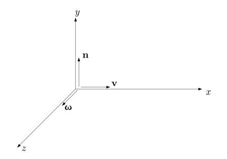
Figure 7.18: Coordinate system aligned with wall streamlines and vortex lines.
