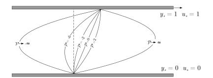
Figure 10.7: Velocity profiles for various values of  $\mathcal{P}$  for Couette flow with pressure gradient.
