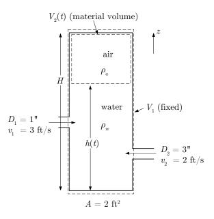
Figure 4.7: Sketch of volume with water and air being filled with water.
