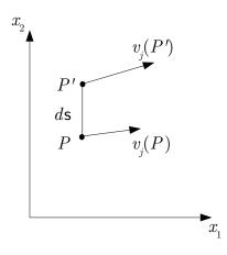
Figure 3.7: Sketch of fluid particle at P and P' in motion.
