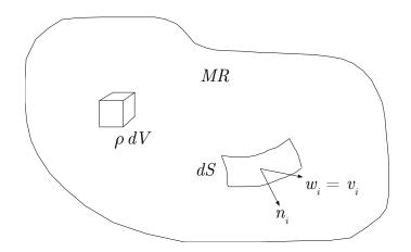
Figure 4.1: Sketch of finite material region MR, infinitesimal mass element  $\rho \, dV$ , and infinitesimal surface element dS with unit normal  $n_i$ , and general velocity  $w_i$  equal to fluid velocity  $v_i$ .
