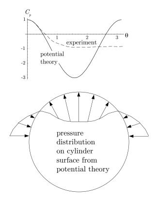
Figure 9.17: Pressure distribution for ideal flow over a cylinder without circulation.
