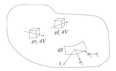
Figure 4.2: Sketch of finite material region MR, infinitesimal linear momenta element  $\rho v_i \, dV$ , infinitesimal body force element  $\rho f_i \, dV$ , and infinitesimal surface element dS with unit normal  $n_i$ , surface traction  $t_i$  and general velocity  $w_i$  equal to fluid velocity  $v_i$ .
