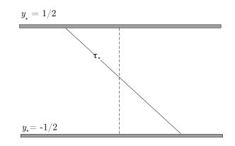
Figure 10.4: Shear stress profile for pressure gradient-driven flow in a slot.
