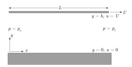
Figure 10.6: Configuration for Couette flow with pressure gradient.
