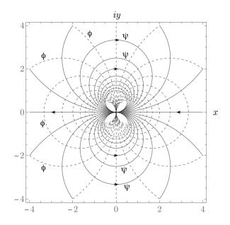
Figure 9.14: Streamlines and equipotential lines for a doublet. Notice because the sink is infinitesimally to the right of the source, there exists a directionality. This can be considered a type of *dipole moment*; in this case, the direction of the dipole is  $-\mathbf{i}$ .
