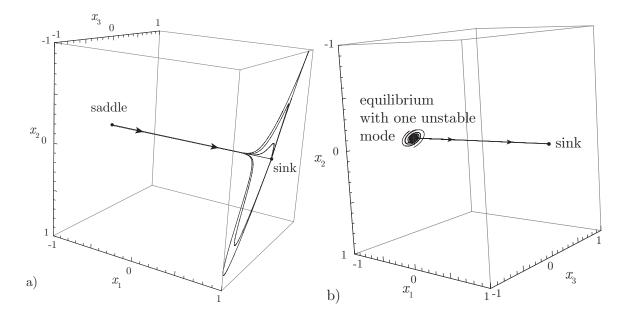
Figure 3.18: Plots of trajectories near the heteroclinic connection between equilibria with one unstable mode and a sink illustrating a) divergence of nearby trajectories due to positive normal stretching with insufficiently rapid rotation and b) convergence of nearby trajectories in the presence of positive normal stretching with sufficiently rapid rotation.
