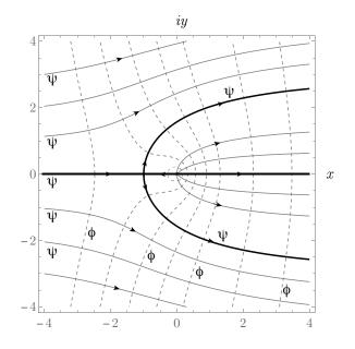
Figure 9.15: Streamlines for a Rankine half body.
