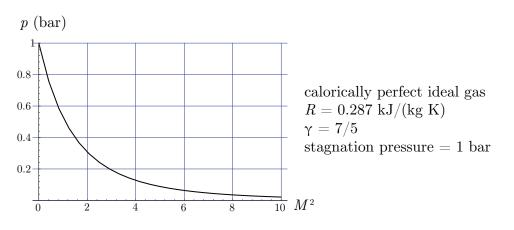
Figure 8.3: Static pressure versus Mach number squared.
