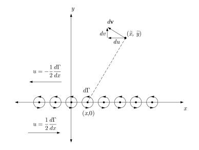
Figure 7.14: Sketch showing schematic of vortex sheet.
