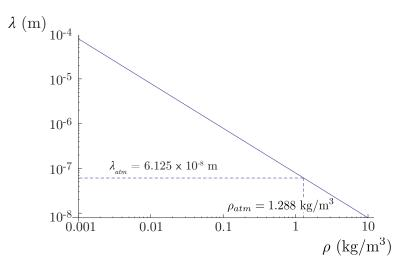
Figure 1.2: Mean free path length,  $\lambda$ , as a function of density,  $\rho$ , for air.
