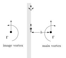
Figure 7.13: Sketch showing a vortex and its image to simulate an inviscid wall.
