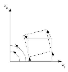
Figure 3.9: Sketch of pure rigid body rotation.
