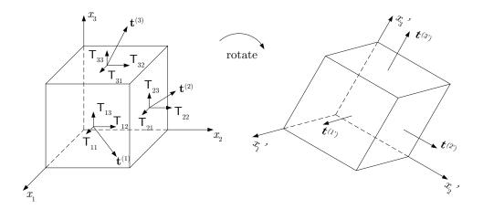
Figure 2.3: Sample Cartesian element that is rotated so that its faces have vectors that are aligned with the unit normals associated with the faces of the element.
