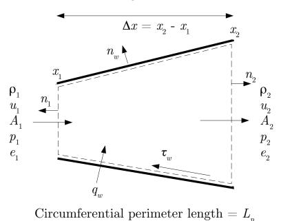
Figure 8.1: Control volume sketch for one-dimensional compressible flow with area change, heat transfer, and wall friction.
