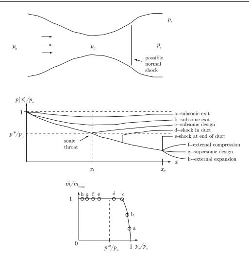
Figure 8.14: Converging-diverging nozzle sketch.
