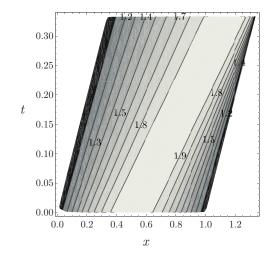
Figure 8.28: Early time solution to  $\partial u/\partial t + u\partial u/\partial x$  with  $u(x,0) = 1 + \sin \pi x$  in the form of a contour plot in x - t space giving contours of constant u.
