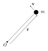
Figure 4.5: Sketch of particle of mass m velocity **v** rotating about an axis centered at point O, with radial distance vector **r**.
