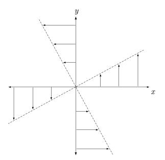
Figure 7.4: Sketch of a fluid rotating as a pure solid body.
