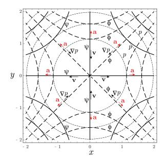
Figure 9.10: Sketch for  $W(z) = z^2$  of streamlines, equipotential lines, isobars, velocity vectors, acceleration vectors, pressure gradient vectors.
