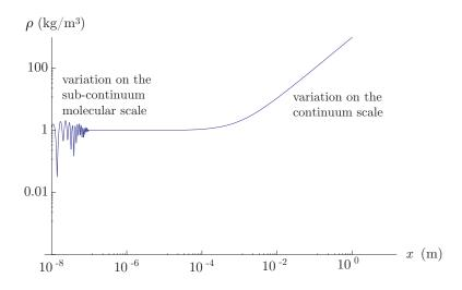
Figure 1.1: Sketch of possible density variation of a gas near atmospheric pressure.
