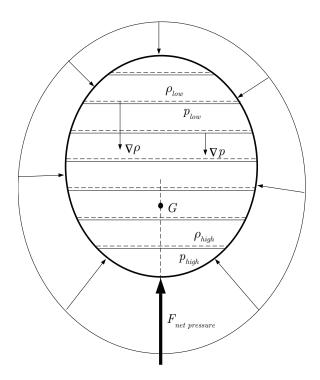
Figure 7.6: Isobars and isochores, center of mass G, and center of pressure for a barotropic fluid.
