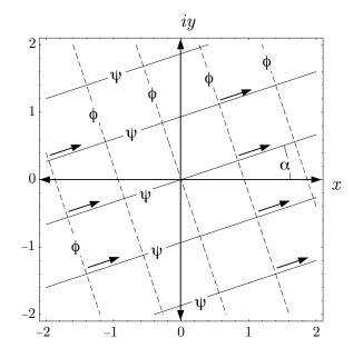
Figure 9.5: Streamlines and equipotential lines for uniform flow.
