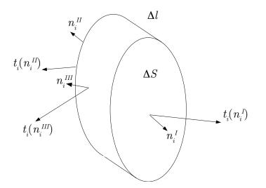
Figure 4.3: Sketch of pillbox element for stress analysis.
