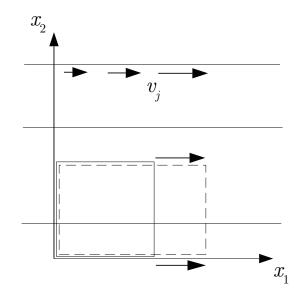
Figure 3.10: Sketch of extensional flow (1-D compressible).
