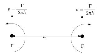
Figure 7.12: Sketch showing a pair of counterrotating vortices of equal strength.
