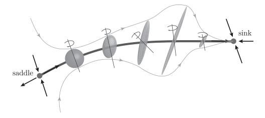
Figure 3.17: Sketch of a phase volume with  $\nabla^T \cdot \mathbf{v} < 0$  showing heteroclinic connection between a saddle and sink equilibria along with the evolution of a set of points initially configured as a sphere as they move into regions with some positive normal stretching rates.
