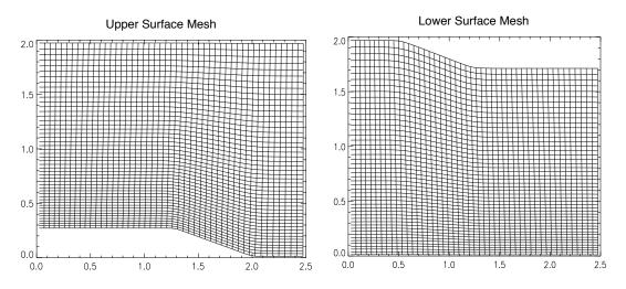
Figure 2: Mesh generated around the diamond shaped airfoil.
