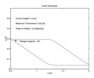
Figure 1: Schematic of diamond shaped airfoil.
