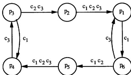
Figure 4: DES Plant of Quasideterministic Double Integrator
