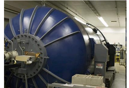
The 10-MV FN Tandem at Notre Dame. Using terminal gas stripping, more than 1 \mu\text{A} ^{13}\text{C} beam was delivered on target.
