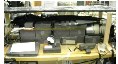
The ^{24}\text{Na} decay counting station consists of two clover detectors, 1 compact plastic \beta -counter and several fiber plastic cosmic ray veto counters.
