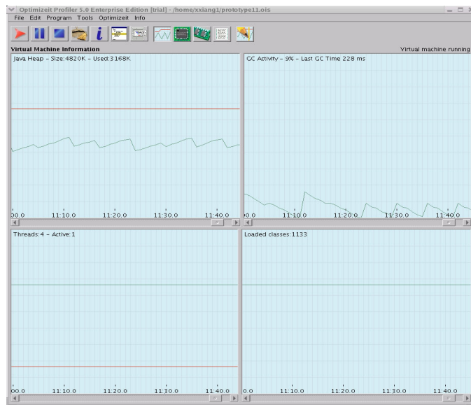
Figure C.3. OptimizIt provides the graph that shows the heap usage, the activation of garbage collector, the thread activity, and the class load information.
