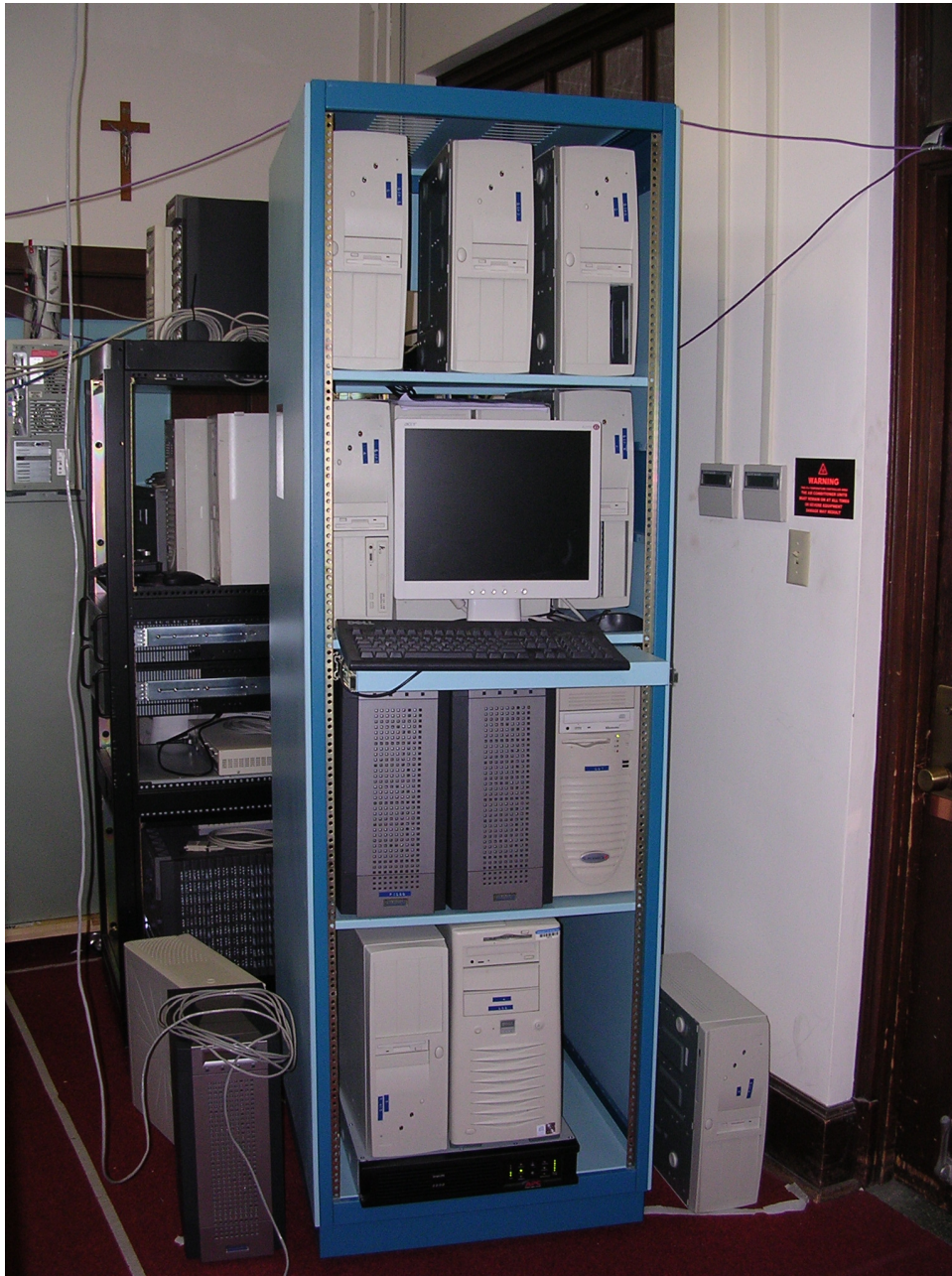
Figure A.1. NOM Cluster of Machines. We have eight simulation machines, a web server, a firewall, and two database machines.
