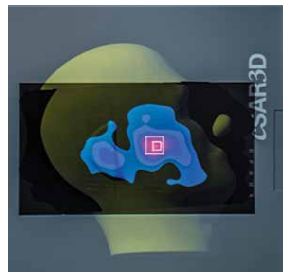
Top: A full-head mannequin testing wireless performance in Notre Dame's anechoic chamber. Center photos: Electromagnetic "heat maps" showing radiation emitting from a phone. Researchers seek to improve phone performance, while keeping radiation within safe limits.
