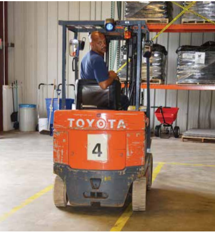
Material handler Wayne Batteast demonstrates a forklift outfitted with a new backup safety light system.
