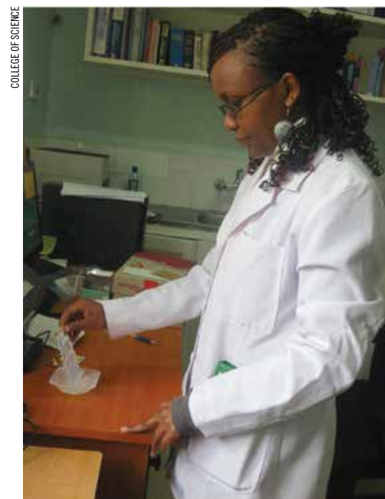
A Kenyan pharmacist uses a paper analytical device to test for counterfeit drugs.
