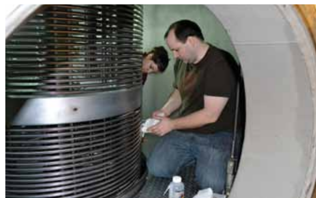
Postdoc Dan Robertson and graduate student Stephanie Lyons work on the final cleaning of the hoops inside the accelerator, in preparation for closing the tank. Air will be pumped out and the tank filled with sulfur hexafluoride ( SF_6 ), an inert gas that will allow the maintenance of a stable 5 million volts.
