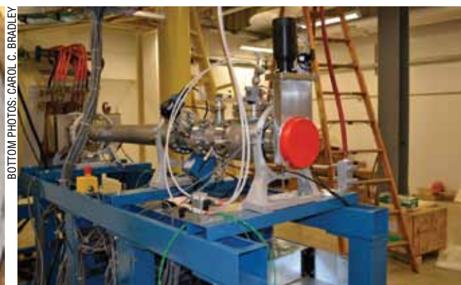
The accelerator will generate electrical potentials up to 5 million volts. Then a gas is ionized in the terminal by removing electrons, resulting in a +2 or +3 charge state. “Since like charges repel each other, ions are accelerated out of the terminal and toward the magnet,” says Ed Stech, associate professional specialist.
