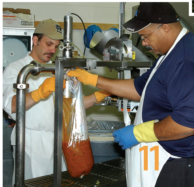
11. Bloss and Dokes pump the finished product—at a temperature of 180 degrees—from the kettle into 75 two-gallon plastic bags, which are sealed, stapled and labeled.
