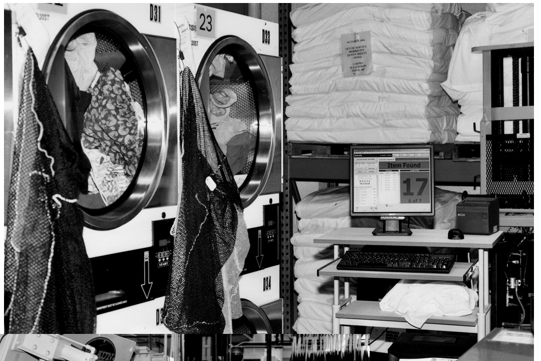
Above: The laundry has a computerized bar-code system for washing and drying student laundry. Students no longer have to mark individual items.
