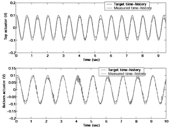
Fig. 9. Sinusoidal load simulation with actuator frequencies: Top—1.5 Hz and bottom—1.0 Hz
