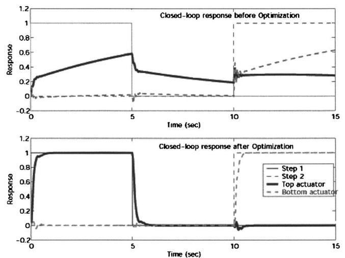
Fig. 7. Closed loop response of two outputs to sequential step loading prior to and after optimization
