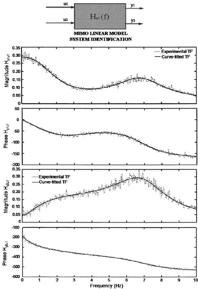
Fig. 5. Open loop transfer functions (experimental and curve fitted)
