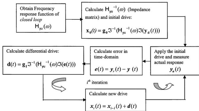
Fig. 3. Iterative scheme for multiactuator control
