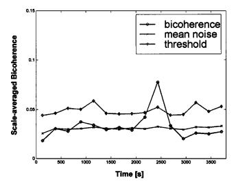
Fig. 14. Scale-averaged bicoherence of experimental tension leg offshore platform data
