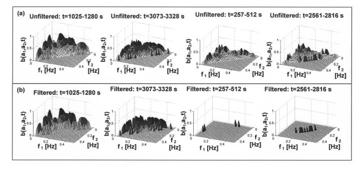
**Fig. 11.** Wavelet bicoherence maps between  $v_1(t)$  and pr(t): (a) unfiltered and (b) filtered. Signals are correlated over 1,025–1,280 s and 3,073–3,328 s, uncorrelated over 257–512 s and 2,561–2,816 s
