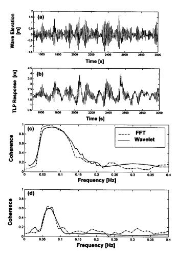
**Fig. 2.** (a) Incoming wave surface elevation; (b) tension leg offshore platform surge response; (c) wavelet and fast Fourier transform coherence estimates between wave elevation and tension leg offshore platform response; and (d) wavelet and FFT coherence estimates between wave elevation and tension leg offshore platform response with incoherent noise added to each
