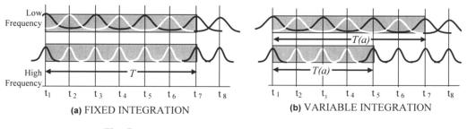
**Fig. 5.** Illustration of variable integration window concept
