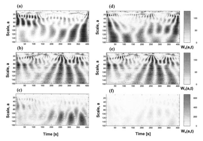
**Fig. 1.** (a) Scalogram of upstream wind velocity 1; (b) scalogram of rooftop pressure; (c) coscalogram of these two correlated processes; (d) scalogram of upstream wind velocity 2; (e) scalogram of rooftop pressure; and (f) coscalogram of these two uncorrelated processes
