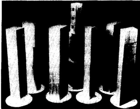
Fig. 2: Models of High-Rise Buildings for Force Balance Study
