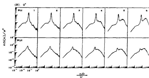
Fig. 5: Pressure Spectra on Side Face
