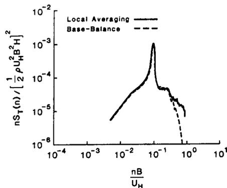
Fig. 9: Torsional Load Spectra Utilizing Pneumatic Averaging and Force Balance Techniques
