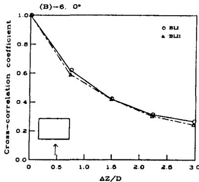
Fig. 7: Spanwise Correlation Near Downwind End
