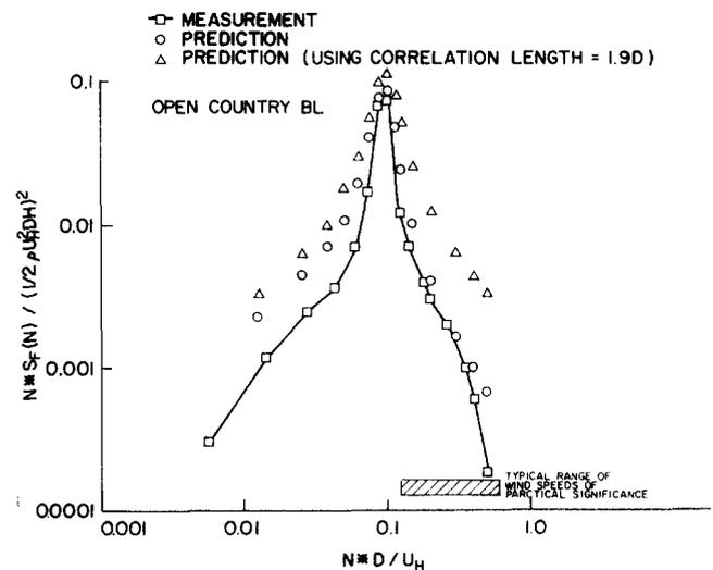
Figure 4 Predicted and measured mode-generalized spectra for open country flow
