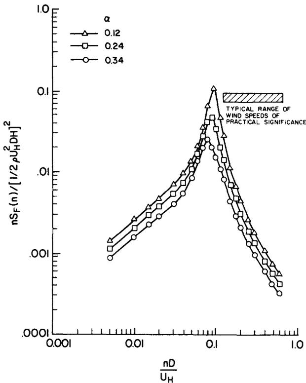
Figure 6 Mode-generalized spectra for open country, suburban and urban flow conditions
