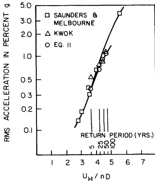
Figure 9 Comparison of predicted and experimental rms acceleration response
