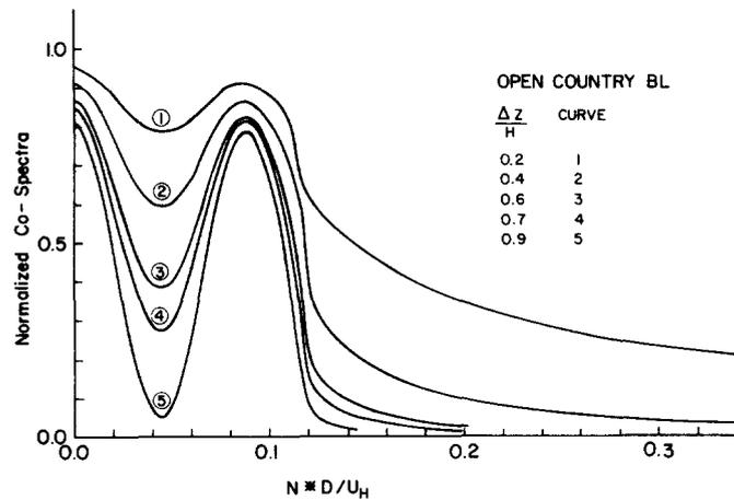
Figure 2 Normalized predicted co-spectra for open country flow
