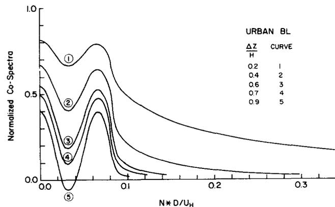
Figure 3 Normalized predicted co-spectra for urban flow
