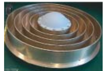
ANTENNA with four concentric choke rings to allow operations in a dense urban zone populated by reflective surfaces
