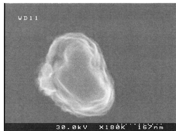
FIG. 5. SEM of an Al nanodot produced by depositing through a polyimide membrane mask.
