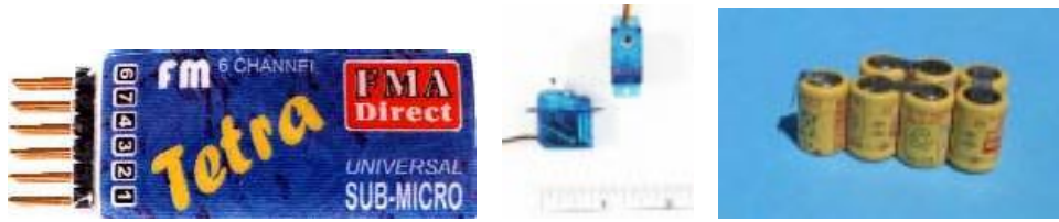
Figure 6: Radio Control Receiver, Servos, and NiCd batteries
