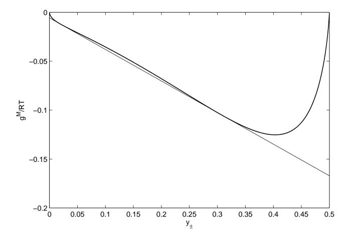
Figure 2: Gibbs energy versus composition surface for eNRTL ( $\rho=25$ ) with parameter solution 2 (see Table 5) for the [bmpy][Tf<sub>2</sub>N] and n-hexanol system. The bitangent line represents the experimental LLE at  $y_{\pm, \rm exp}^{\rm I}=0.0202$  and  $y_{\pm, \rm exp}^{\rm II}=0.3080$ .
