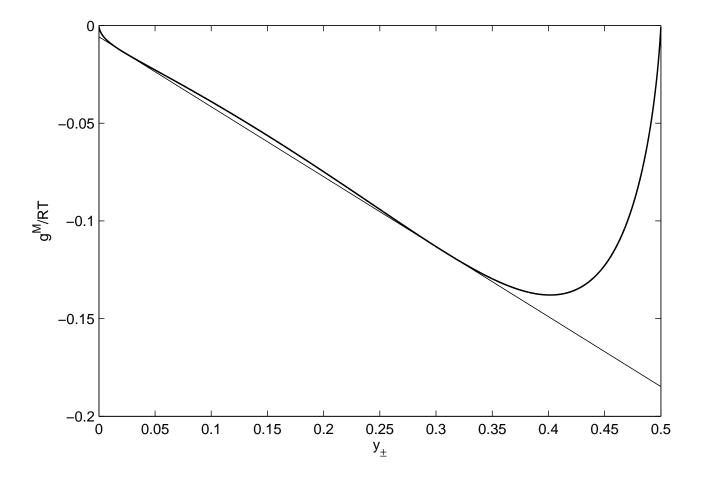
Figure 3: Gibbs energy versus composition surface for eNRTL ( $\rho=25$ ) with parameter solution 3 (see Table 5) for the [bmpy][Tf<sub>2</sub>N] and n-hexanol system. The bitangent line represents the experimental LLE at  $y_{\pm, \rm exp}^{\rm I}=0.0202$  and  $y_{\pm, \rm exp}^{\rm II}=0.3080$ .
