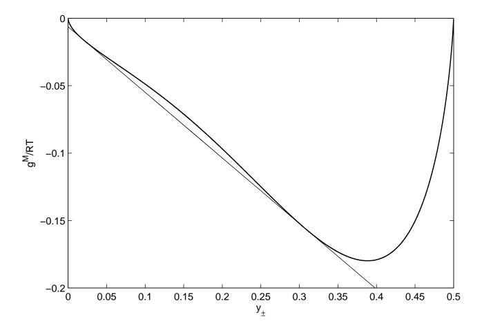
Figure 1: Gibbs energy versus composition surface for eNRTL ( $\rho=25$ ) with parameter solution 1 (see Table 5) for the [bmpy][Tf<sub>2</sub>N] and n-hexanol system. The bitangent line represents the experimental LLE at  $y_{\pm, \rm exp}^{\rm I}=0.0202$  and  $y_{\pm, \rm exp}^{\rm II}=0.3080$ .
